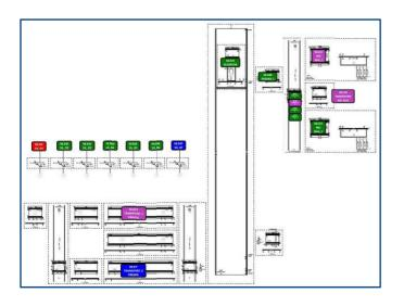
The factory overview software is programmed in the MTD Fat Client. The status of a machine is visible. Which allows immediate intervention. The status of machines/equipment is visualised with a push button. Each colour has a meaning. As soon as the button is pressed, an extra screen will be shown where any malfunction is located, with all documents visualised.
