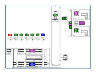
The factory overview software is programmed in an MTD Fat Client. The status of a machine is visible. Allowing immediate intervention. The status of machines/equipment is visualised with a push button. Each colour has a meaning. As soon as the button is pressed, an extra screen will be shown where any malfunction is located, with all documents visualised.
