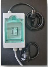
The MTD Load indicator, is directly linked to the MTD Master-/ Slave Module. With this indicator the load of a device / machine is read out and sent to the MTD Control Module.
